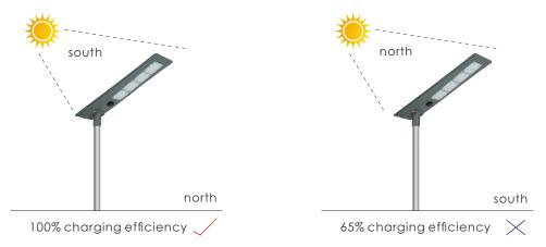
(A diagram for how the orientation impacts on power generation efficiecy)
