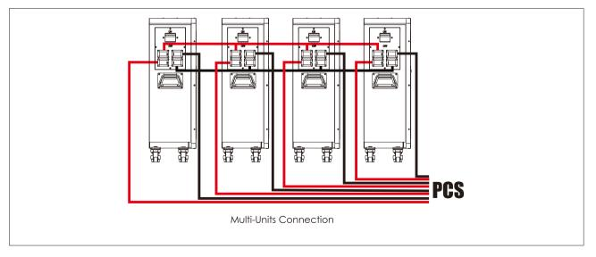
Master Pack and Slave Pack can be used as single unit as well as multi-units (in parallel)mode.
