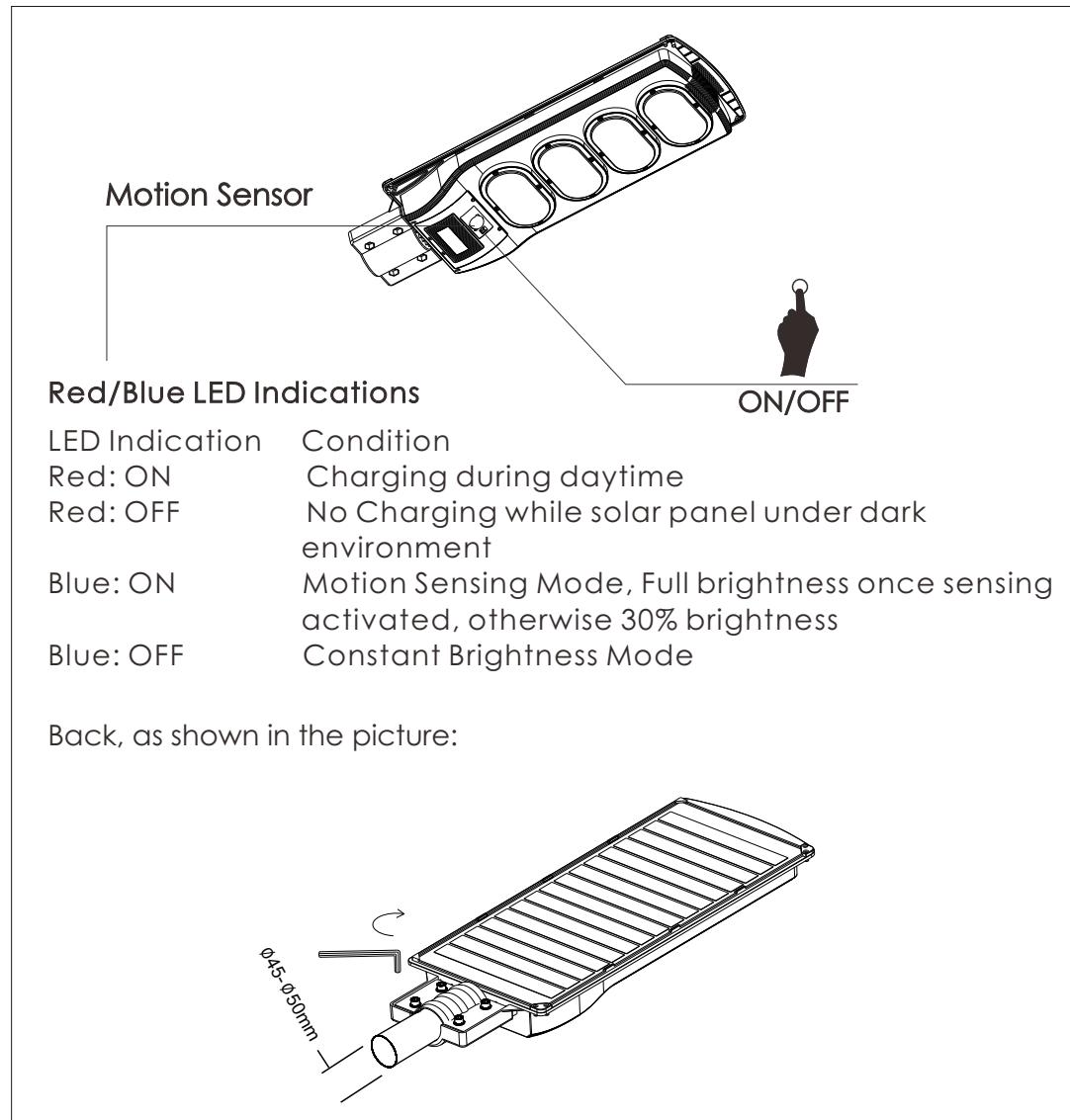
1. Insert the lamp arm into the lamp body and tighten the screw.
